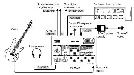
**NOTE:** Since ToneLab uses an actual valve (vacuum tube), it will produce no sound for several seconds until the valve warms up. This isn't a malfunction - it's just the nature of valves.
